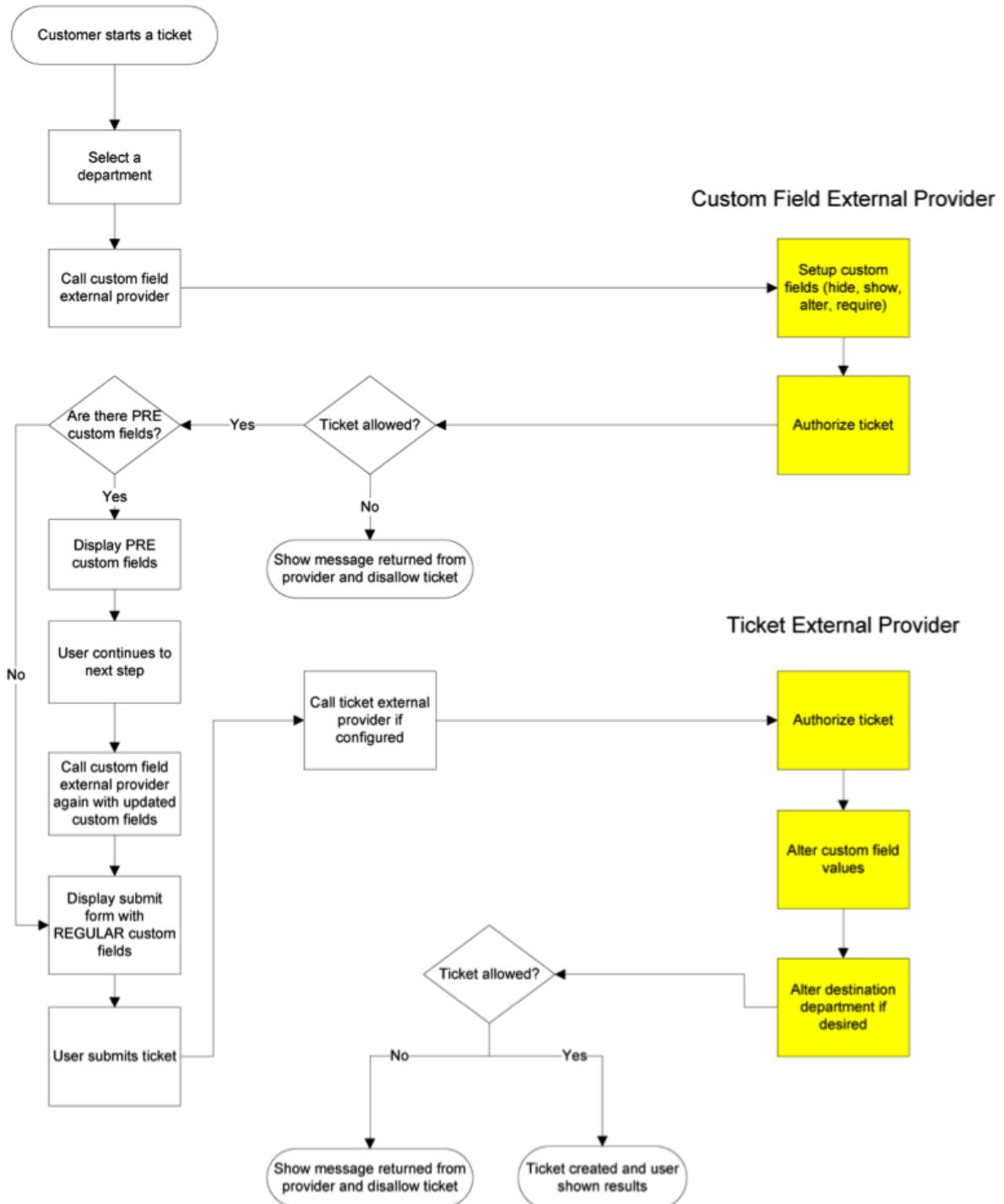
In the example below, the custom field provider is used to determine the options available on each step in the ticket submission process and the ticket tracking provider uses the options selected to determine whether the ticket can be started.
